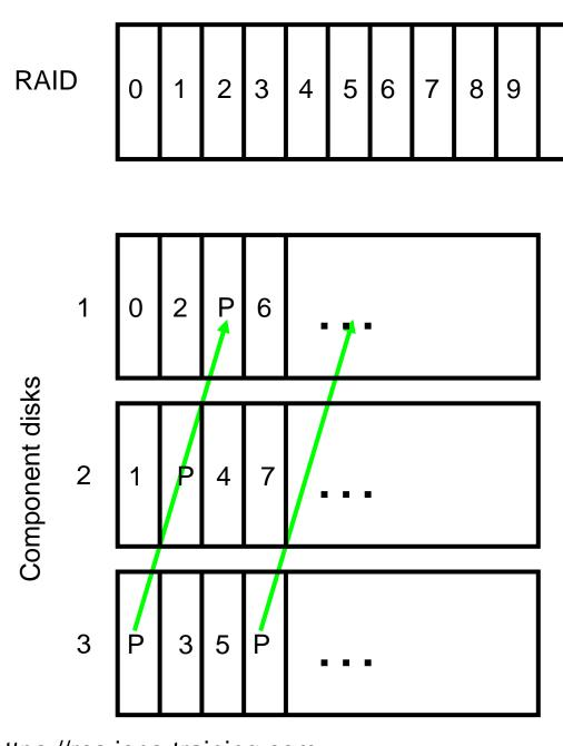
backward parity aka left asymmetric (used in Adaptec chip sets)
